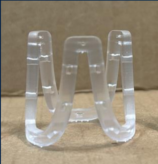
3-D printed coronet-shaped rigid ring
